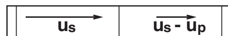
FIG. 1. A stationary one-dimensional shock wave. Cold material enters at the left with a speed u_s , passes through the shock front which separates the cold material from the hot, and exits at the right with speed u_s - u_p . The cold-to-hot conversion process is irreversible and corresponds to an overall entropy increase.
